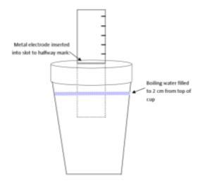
4. Before filling cup with boiling water, set up the cup with lid and metal electrode and have students use the infrared thermometer to measure the temperature of the metal electrode at each of the centimeter marks. Data should be recorded at Time=0 minutes in a chart similar to the example:
